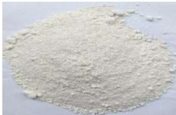
Fig 2. Egg shell Powder used in Concrete
